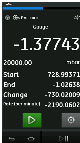
Figure 2-24: Leak Test Example
