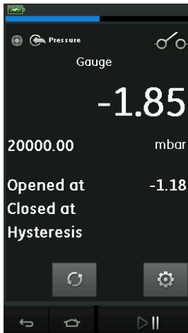
Figure 2-14: Switch Test Example
