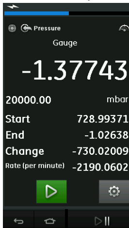
Figure 2-26: Leak Test Example
